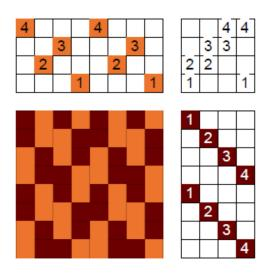
We can "break" the straight twill line by reversing any two shafts. I prefer the break to occur with shafts 2 and 3, as shown on the left to avoid floating selvages by preserving the starting shaft at 1 and the ending shaft at 4 (then enter the shuttle on the side of the warp where the first thread is down).
